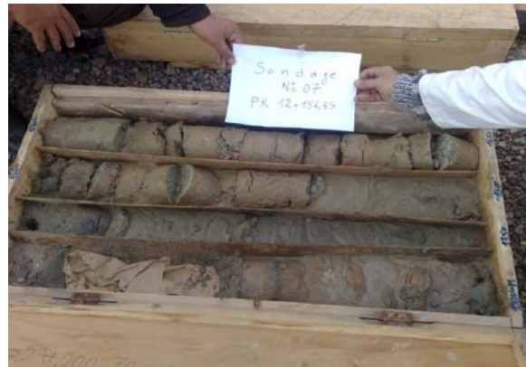
Figure 3: Bore hole soil samples
