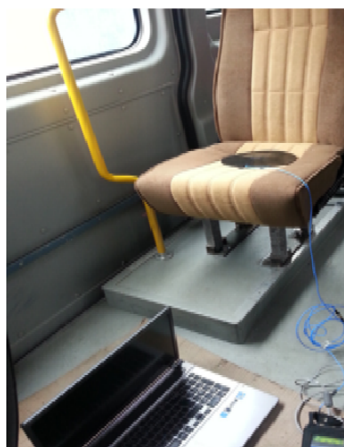
Figure 2 Acceleration measurement test work
